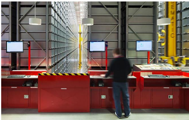
Figure 6: Automated Storage and Retrieval System (ASRS), or BookBot
