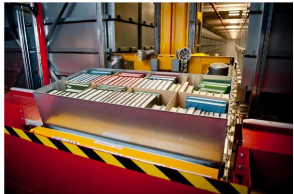
Figure 6: Automated Storage and Retrieval System (ASRS), or BookBot
